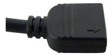
This arrow must match with the 12v pin for the system to receive power. The power draw per foot is ~2.16w, meaning the max length of a single run is determined by the transformer. The max length of a 24w transformer is 11 feet and the max for a 40w transformer is 18.5 feet.
