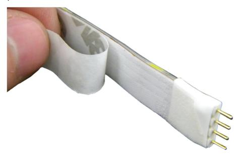
When connecting the first strip in a run to power, it is important to get the polarity in line with the strip configuration. Looking closely at the strip, you will be able to notice the designation of the pins. Starting at the top, the pin configuration is B R G 12V.
